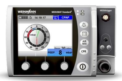
CPAP mode, which allows for the patient's spontaneous breathing at an increased pressure level, has proven itself in treatment of cardiac pulmonary edema\*\*. CPAP pressure can be finely adjusted anytime with MEDUMAT Standard<sup>2</sup>. The device recognizes and compensates for leakage at the mask. During ventilation all parameters can be adjusted via the monitor.
